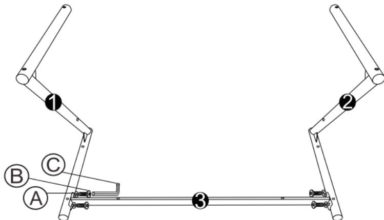
Please note, washers should be turned with the concave side to the table leg, and the curved side to the bolt.
