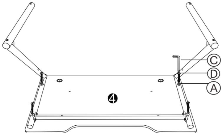
Please note, washers should be turned with the concave side to the table leg, and the curved side to the bolt.
